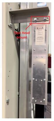
Once the bracket for the tape head is installed, mount the tape head in the two slotted holes of the bracket using the provided hardware, as shown in Figure 18.
