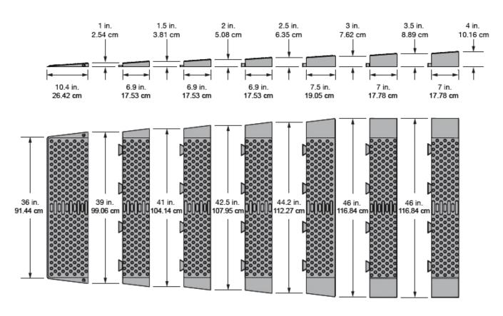
The rubber threshold ramp has a maximum incline of 4° (7%), which meets the requirement established by the ADA.
